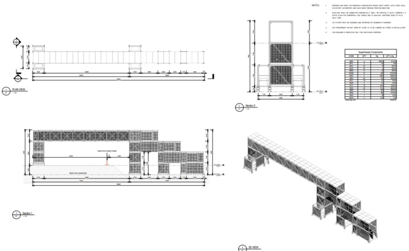
The SuperAccess™ team then built the stair box and bridge at our yard. Preassembling off-site allowed us to install Richard Crookes' temporary access solution in a single day.
